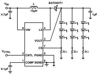
FIGURE 12A. 3 LEGS OF 3 LEDs IN A SERIES
