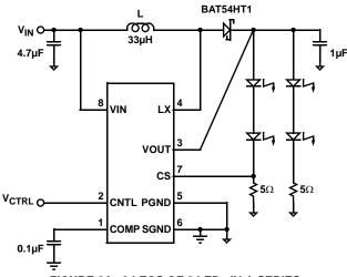
FIGURE 8A. 2 LEGS OF 2 LEDs IN A SERIES
