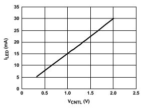
FIGURE 3. I<sub>LED</sub> vs V<sub>CNTL</sub>
