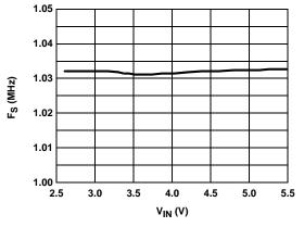
FIGURE 1. SWITCHING FREQUENCY vs VIN
