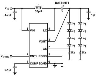
FIGURE 10A. 2 LEGS OF 4 LEDs IN A SERIES
