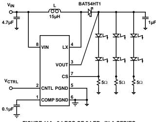
FIGURE 11A. 3 LEGS OF 2 LEDs IN A SERIES
