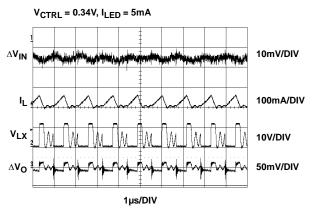
FIGURE 18. DISCONTINUOUS CONDUCTION MODE
