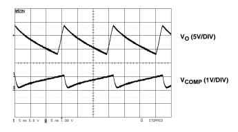
FIGURE 19. OVER VOLTAGE PROTECTION (LED DISCONNECTED)
