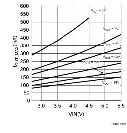
FIGURE 18. Typical Maximum Output Current in OLED Mode (assumed 80% efficiency)
