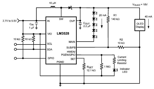
OLED Panel Power Supply With Indicator LED
