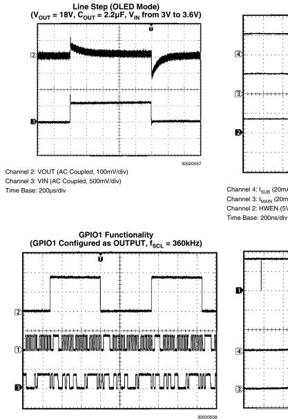
Channel 2: GPIO (2V/div) Channel 1: SCL (5V/div) Channel 1:SDA (5V/div) Time Base: 40µs/div
