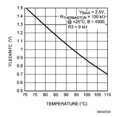
FIGURE 24. Thermistor Resistive Divider Response vs Temperature
