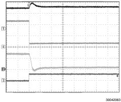
**Line Transient** (LED Mode, Single LED,  $I_{FLASH} = 1.2A$ )
