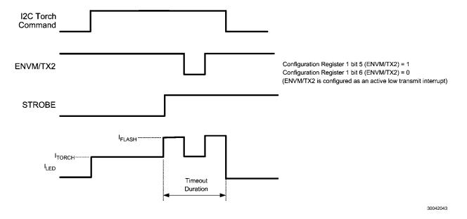
FIGURE 9. ENVM/TX2 Pin is Configured as an Active Low TX Input
