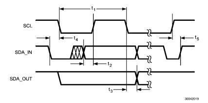
FIGURE 14. I<sup>2</sup>C-Compatible Timing
