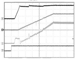
Channel 1:  $V_{OUT}$  (2V/div) Channel 4:  $I_{LED}$  (500mA/div) Channel 2:  $I_{L}$  (500mA/div) Channel 3: STROBE (5V/div) Time Base: (100 $\mu$ s/div)
