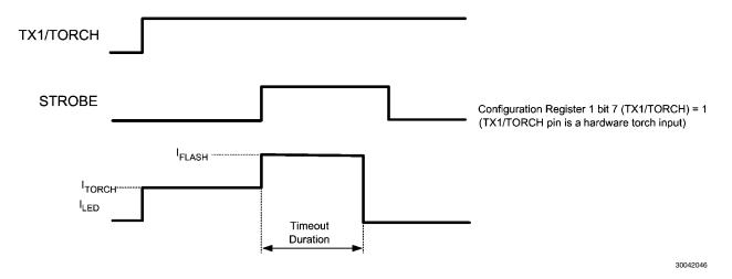
FIGURE 12. TX1/TORCH Configured as a Hardware Torch input
