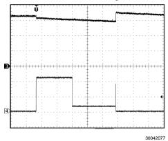
Channel 3: V<sub>IN</sub> (1V/div) Channel 4: I<sub>LED</sub> (500mA/div) Time Base: (100ms/div)
