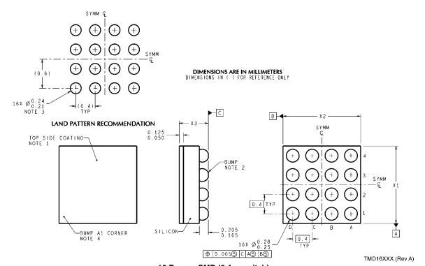
16 Bump  $\mu$ SMD (0.4mm pitch) For Ordering, Refer to Ordering Information Table NS Package Number TMD16CCA X1 = 1.695mm (±0.03mm), X2 = 1.695mm (±0.03mm), X3 = 0.6mm(±0.075mm)
