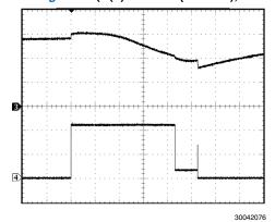
Channel 3: NTC Pin Voltage (500mV/div)
