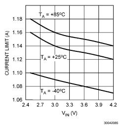
Shutdown Current vs  $V_{IN}$ ( $V_{HWEN} = 0V$ )
