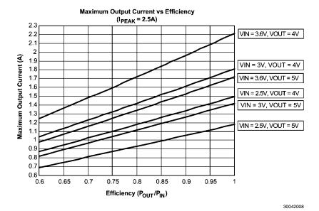
FIGURE 2. LM3554 Maximum Output Current
