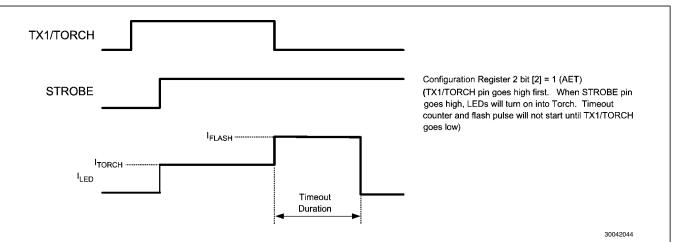
FIGURE 10. Alternative External Torch Mode (TX1/TORCH Turns on Before STROBE)
