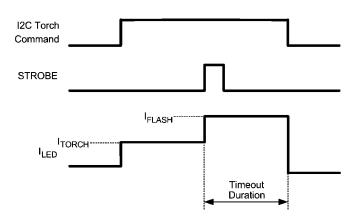
Flash Brightness Register bit 7 (STR) = 1 STROBE goes high and the LEDs turn on into Flash mode. LEDs will stay on for the timeout duration even if STROBE goes low before.
