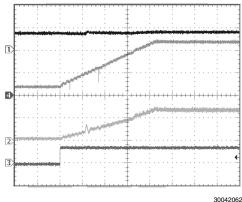
Channel 1: V<sub>OUT</sub> (2V/div) Channel 4: I<sub>LED</sub> (500mA/div)
