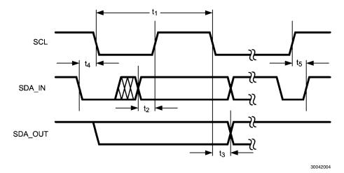
FIGURE 1. I<sup>2</sup>C Timing
