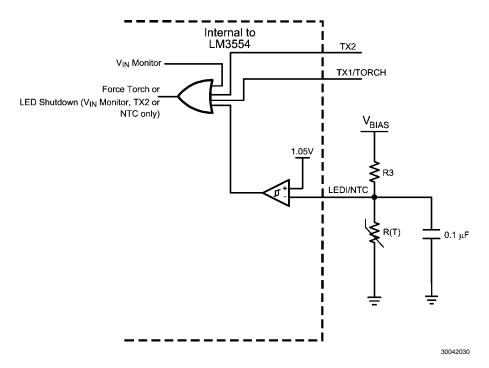
FIGURE 25. Thermistor Voltage Divider and Sensing Circuit
