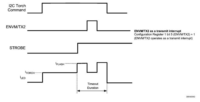
FIGURE 8. ENVM/TX2 Pin is Configured as an Active High TX Input
