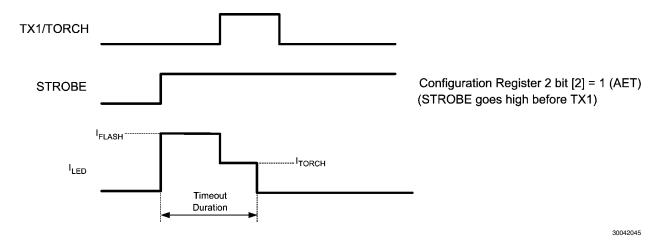
FIGURE 11. Alternative External Torch Mode (STROBE Goes High Before TX1/TORCH, Same as Default with SEM = 0)
