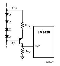
FIGURE 11. Floating Output OVP Circuitry
