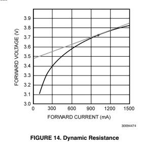
Obtaining  $r_{LED}$  is accomplished by refering to the manufacturer's LED I-V characteristic. It can be calculated as the slope at the nominal operating point as shown in *Figure 14*. For any application with more than 2 series LEDs,  $R_{SNS}$  can be neglected allowing  $r_D$  to be approximated as the number of LEDs multiplied by  $r_{LED}$ .
