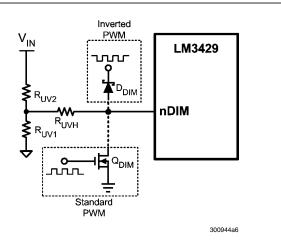
FIGURE 13. PWM Dimming Circuit
