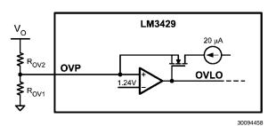
FIGURE 10. Over-Voltage Protection Circuitry
