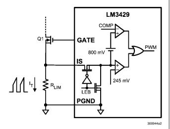
FIGURE 6. Current Sense / Current Limit Circuitry
