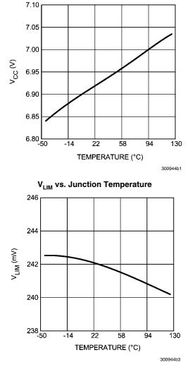
V<sub>CC</sub> vs. Junction Temperature
