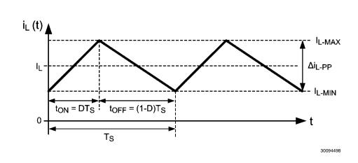
FIGURE 1. Ideal CCM Regulator Inductor Current i<sub>1</sub>(t)
