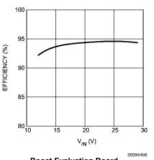
Boost Evaluation Board 9 Series LEDs at 1A
