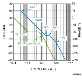
FIGURE 9. Compensated Loop Gain Frequency Response
