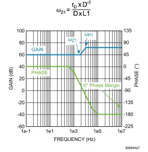
FIGURE 7. Uncompensated Loop Gain Frequency Response
