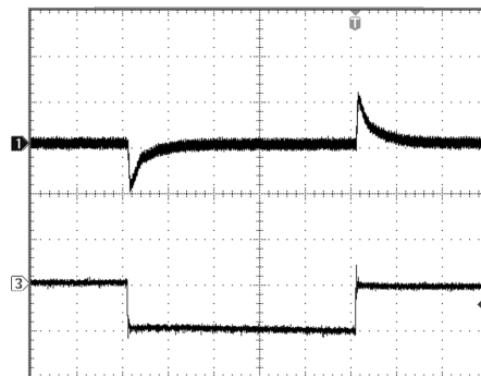
Line Step (LED Mode) (2 × 5 LEDs, 30mA per String, C_{OUT} = 1\mu F )
