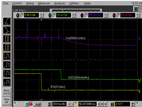
FIGURE 17. ISL97675 SHUTS DOWN AND STOPS SWITCHING ~ 30ms AFTER EN GOES LOW
