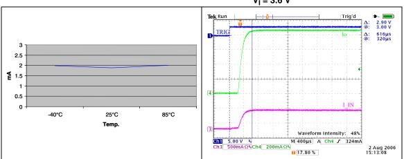
Figure 21.  $I_Q$  vs. temp.  $V_I$  = 5.5 V ready-mode Figure 22. Start-up in flash mode 800 mA at  $V_I$  = 3.6 V
