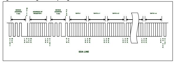
Figure 12. Reading from multiple registers
