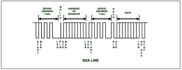
Figure 11. Reading from a single register
