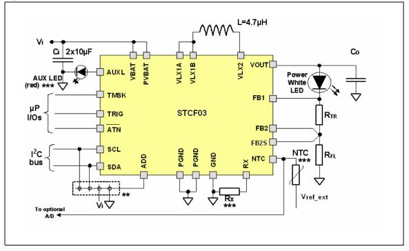
Figure 3. Application schematic
