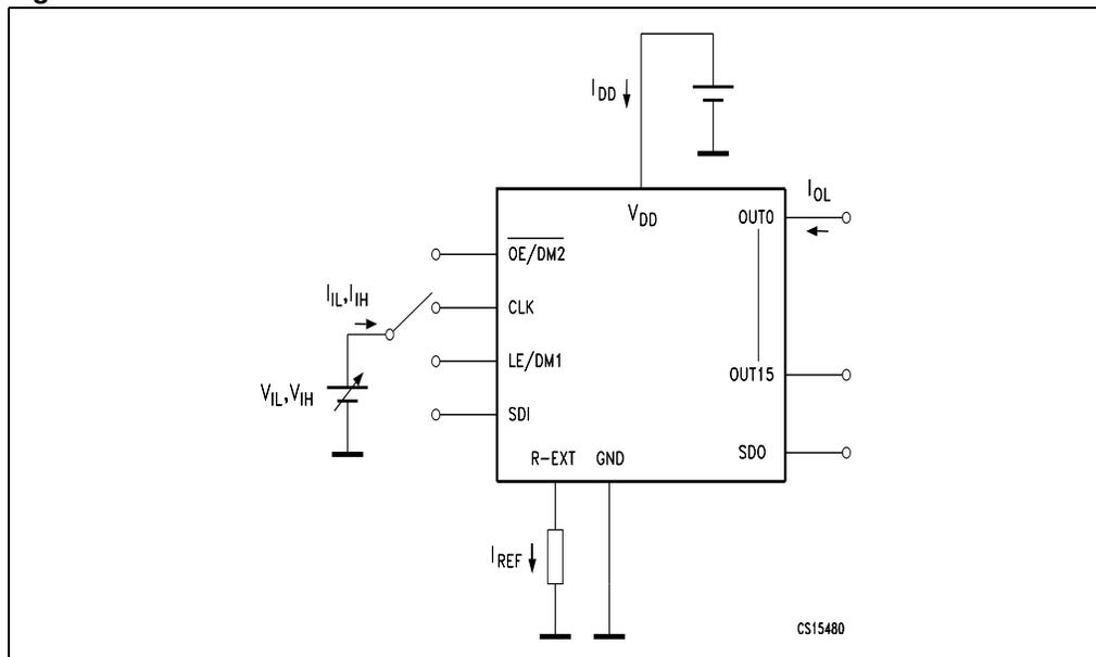
Figure 18. Typical application schematic
