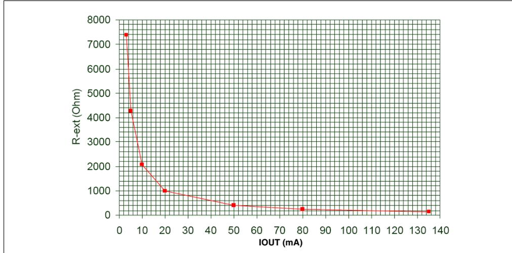
Table 10. Output current- $R_{EXT}$  resistor
