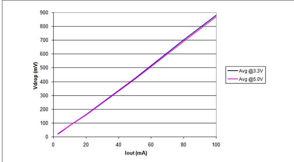
Table 11.  $I_{SET}$  vs drop out voltage ( $V_{drop}$ )
