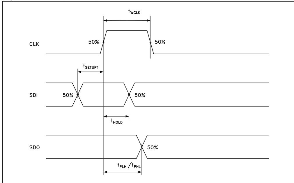
Figure 10. Clock, serial-in, latch, enable, outputs
