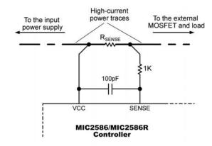
Figure 9. Current Limit Sense Filter for Noisy Systems
