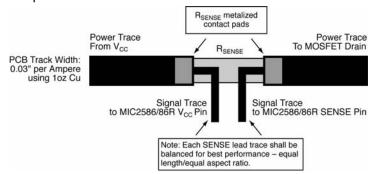
Figure 8. 4-Wire Kelvin Sense Connections for R<sub>SENSE</sub>
