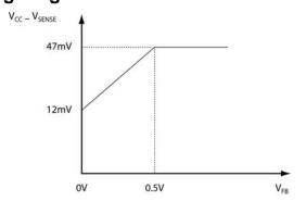
Figure 1. Foldback Current Limit Transfer Characteristic
