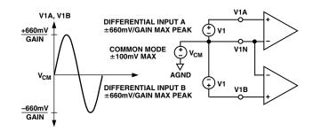
Figure 5. Maximum Signal Levels, Channel 1
