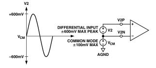
Figure 4. Maximum Signal Levels, Channel 2
