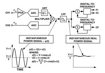
Figure 2. Signal Processing Block Diagram
