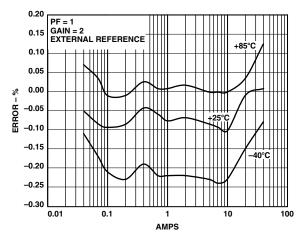
TPC 9. Error as a % of Reading over Temperature with an External Reference (Gain = 2)
