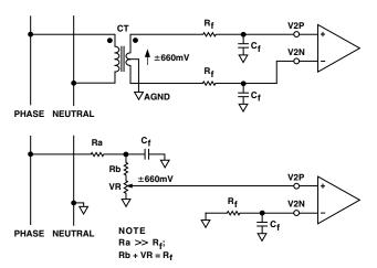
Figure 7. Typical Connections for Channel 2
