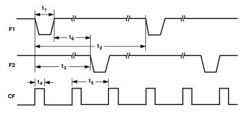
Figure 1. Timing Diagram for Frequency Outputs
