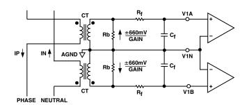
Figure 6. Typical Connection for Channel 1
