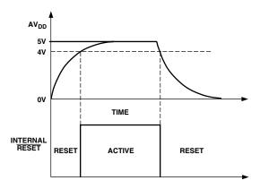
Figure 8. On-Chip Power Supply Monitor
