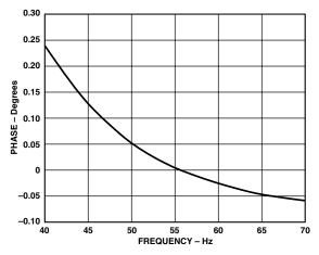
Figure 11. Phase Error Between Channels (40 Hz to 70 Hz)
