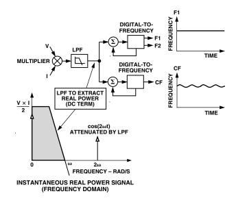
Figure 12. Real Power-to-Frequency Conversion
