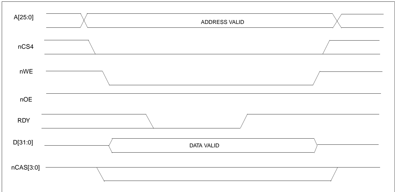
Figure 2-2: SA-1110 Variable-Latency IO Write Cycle
