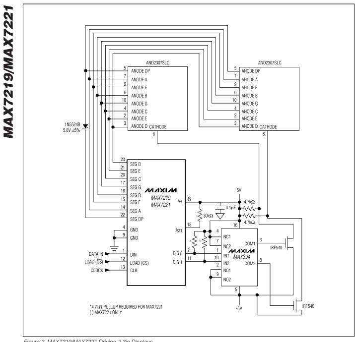
Figure 2. MAX7219/MAX7221 Driving 2.3in Displays
