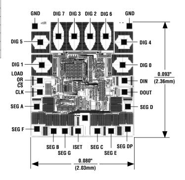
TRANSISTOR COUNT: 5267 SUBSTRATE CONNECTED TO GND
