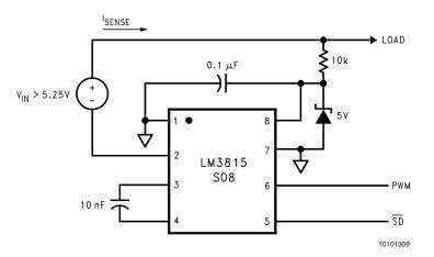
FIGURE 5. High Voltage Operation — V<sub>IN</sub> Greater Than 5.25V (Low Side Sense)
