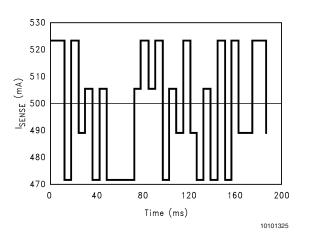
FIGURE 8. Typical Response of LM3814-1.0/LM3815-1.0
