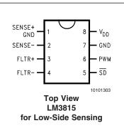
.M3814/LM3815 Fast Current Gauge IC with Ultra Low Loss Sense Element and PWM Output
