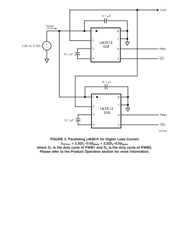
**Typical Application Circuits** In the application circuits, the  $0.1\mu$ F ceramic capacitor between pins 1 and 8 is used for bypassing, and the  $0.1\mu$ F ceramic capacitor between pins 3 and 4 is used for filtering. Shutdown ( $\overline{SD}$ ) is tied to  $V_{DD}$  through a  $10k\Omega$  resistor. (Continued)
