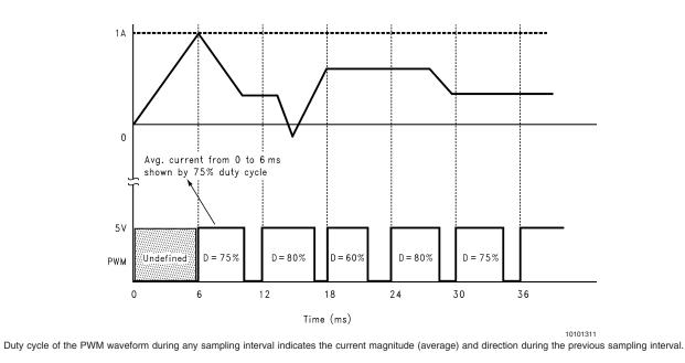
FIGURE 9. Typical Timing Diagram for Mostly Positive Current
