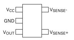
The ZXCT1051 provides a fixed gain of 10 thereby removing the need for an additional resistor.
