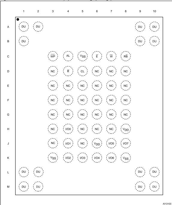
Figure 4. VFBGA63 connections (top view through package)
