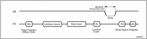
Figure 10. Random data input during sequential data input
