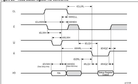
Figure 23. Read status register AC waveforms
