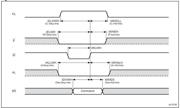
Figure 20. Address Latch AC waveforms
