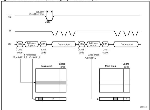
Figure 7. Random data output during sequential data output
