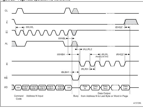
Figure 25. Page read operation AC waveforms
