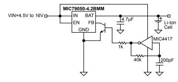
Figure 5B. PWM Based Pulse-charging Applications
