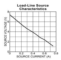
Figure 1B. Load-Line Characteristics of AC Wall Adapter
