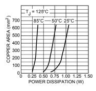
Figure 12. Copper Area vs. Power-MSOP Power Dissipation  $(T_{\Delta})$
