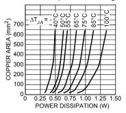
Figure 9. Copper Area vs. Power-SOIC Power Dissipation  $(\Delta T_{J\Delta})$
