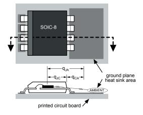
Figure 8. Thermal Resistance
