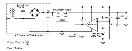
Figure 1A. Load-Line Charger With End-Of-Charge Termination Circuit.
