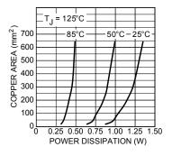
Figure 10. Copper Area vs. Power-SOIC Power Dissipation (T<sub>A</sub>)
