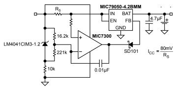
Figure 7. Constant Current, Constant Voltage Charger
