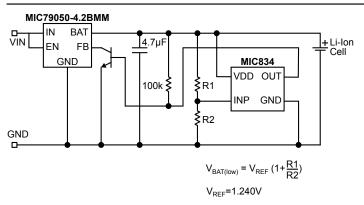
Figure 4. Pulse Charging For Top-off Voltage
