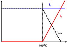
TEMPERATURE FIGURE 8. CURRENT SIGNALS AT THE AMPLIFIER CA INPUT
