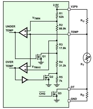
FIGURE 9. THE INTERNAL AND EXTERNAL CIRCUIT FOR THE NTC INTERFACE
