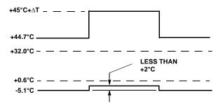
FIGURE 13. BOARD TEMPERATURE MONITORING. WHEN NOT CHARGING, THE TEMPERATURE WINDOW IS BETWEEN -5°C AND +45°C. ONCE THE CHARGER STARTS, THE TEMPERATURE WINDOW IS ~-3°C TO +45°C+ ∆T
