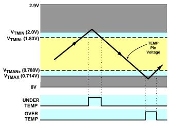
FIGURE 11. CRITICAL VOLTAGE LEVELS FOR TEMP PIN
