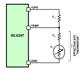
FIGURE 12. EFFECTIVE NTC THERMISTOR CIRCUIT
