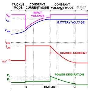
FIGURE 3. TYPICAL CHARGE CURVES USING A CURRENT-LIMITED ADAPTER
