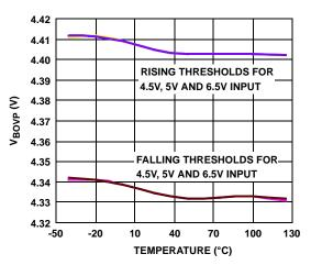
FIGURE 17. BATTERY VOLTAGE OVP THRESHOLDS vs TEMPERATURE AT VARIOUS INPUT VOLTAGES
