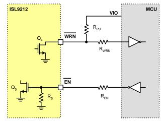
FIGURE 24. DIGITAL SIGNAL INTERFACE BETWEEN ISL9212 AND MCU
