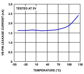
FIGURE 19. VB PIN LEAKAGE CURRENT vs TEMPERATURE
