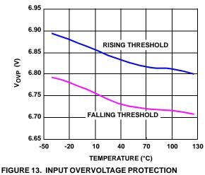
THRESHOLDS vs TEMPERATURE
