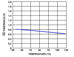
**Typical Operating Performance** The test conditions for the Typical Operating Performance are:  $V_{IN} = 5V$ ,  $T_A = +25^{\circ}C$ ,  $R_{ILIM} = 25.5k\Omega$ ,  $R_{VB} = 200k\Omega$ , Unless Otherwise Noted. (Continued)
