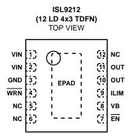
NOTE: EPAD must be electrically connected to the GND pin.
