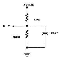
\* INCLUDING SCOPE AND JIG CAPACITANCE
