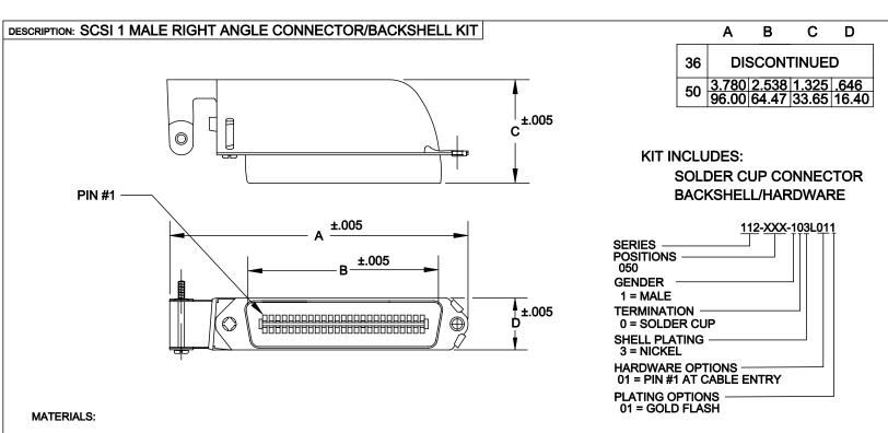
INSULATOR: GLASS-FILLED THERMOPLASTIC UL RATED 94V-0 CONTACTS: COPPER ALLOY SHELL: STEEL, NICKEL PLATED CONTACT PLATING: GOLD PLATED ROHS COMPLIANT
