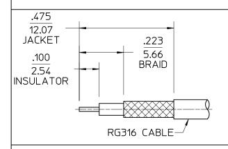
1. STRIP CABLE TO DIMENSIONS SHOWN DO NOT NICK CENTER CONDUCTOR OR BRAID
