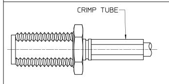
4. SLIP CRIMP TUBE OVER BRAID UNTIL BOTTOMS ON CONNECTOR BODY.
