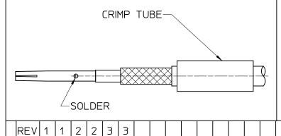
2. SLIP CENTER CONTACT OVER CENTER CONDUCTOR OF CABLE AND SOLDER AS SHOWN.
