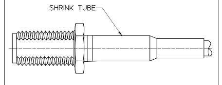
5. SLIP SHRINK TUBE OVER CONNECTOR UNTIL IT BOTTOMS BEHIND THE FLANGE AS SHOWN. APPLY HEAT.
