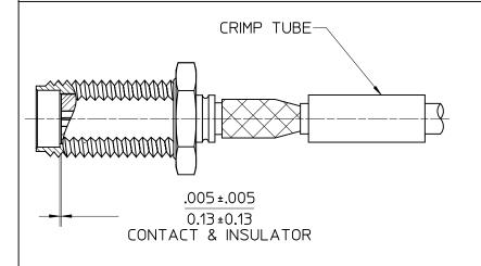
3. FLARE BRAID AND INSERT CABLE INTO CONNECTOR TO DIMENSION SHOWN.
