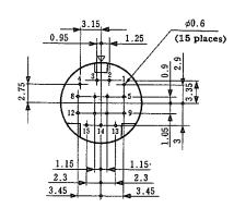
Note: 1. Figures of 13 and 15-conductor connectors are viewing from the mating side of receptacle.
