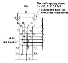
Note: 1. Above figure shows PCB face viewing from the mating face of receptacle.
