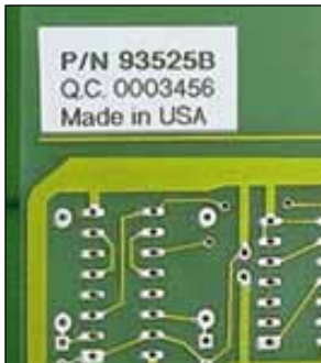
Circuit board labeling
