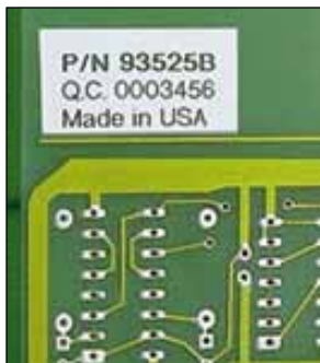
Circuit board labeling
