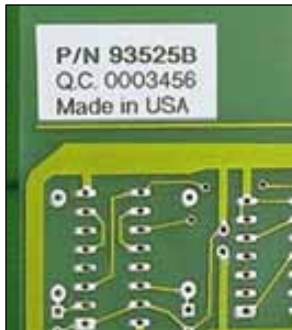
Circuit board labeling
