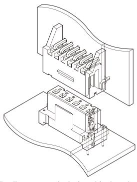
The JL connector is designed for board-toboard connection in electronic equipment requiring high-density mounting and unitization. This connector is highly resistant to equipment vibration and shock.
