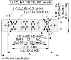
Recommended PCB Thickness  $t=1.6\pm0.19(0.063\pm0.007)$
