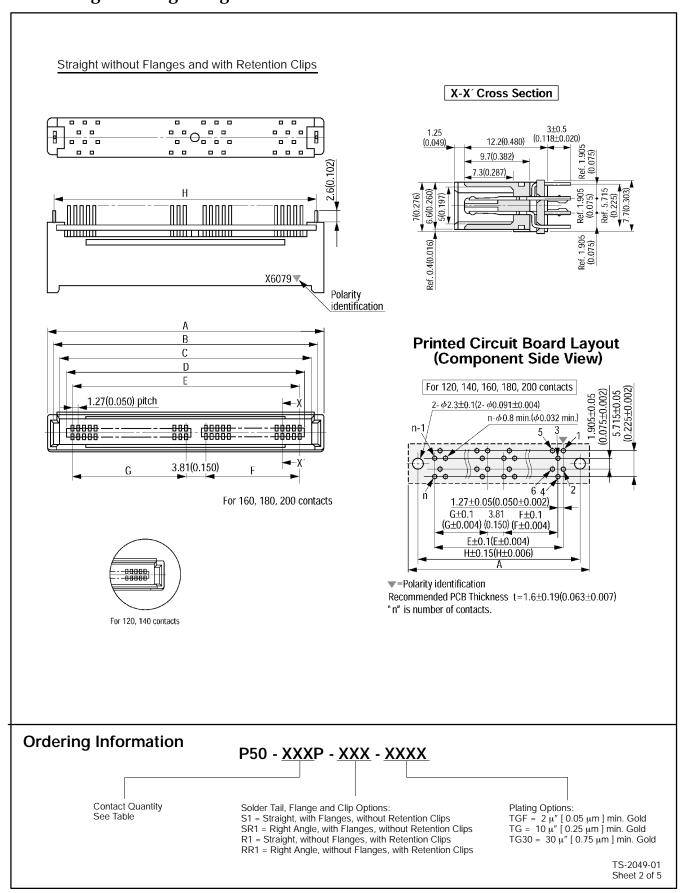
Product Table / Dimensions for Straight and Right Angle without Flanges and with Retention Clips
