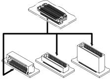
This JMC connector is 0.5mm pitch SMT type board to board connector with selection of boss existence.
