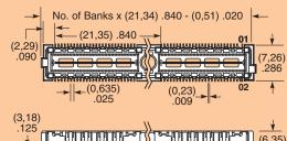
= 10µ" (0,25µm) Gold on Signa Pins, Shield and **Ground Plane** (Gold flash on Signal Pin tails
