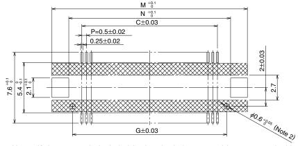
Note1: If the pattern is included in the shaded area, and is not treated with resist, it could touch the connector contact.
