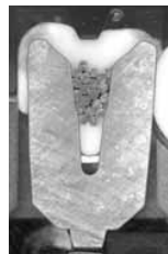
Cross section of wire crimped in the upper tier
