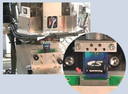
Insertion-removal testing machine testing mis-positioned card insertion in SD socket (mis-positioning correction function) (Joint research with Dr. Toshiro Higuchi of Tokyo University)
