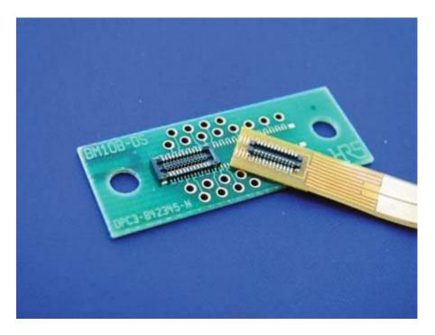
**November 24, 2009 --** Providing design engineers with a versatile, flexible printed circuit connector with minimal board height, <u>Hirose Electric Co., Ltd.</u> has developed a new series of FPC-to-board connectors. Designated the BM10 series, the RoHS-compliant and halogen-free connectors are available with stacking heights of 0.6 mm and 0.8 mm, and feature a space-saving 2.98 mm depth and 0.4 mm contact pitch.
