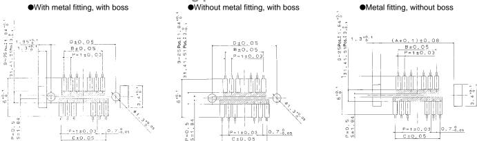
Note 1: [[[]] If the pattern is included in the shaded area and not treated with resist, it could touch the connector contact.
