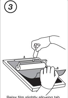
Relax film slightly allowing tab 'A' edge to come close to LCD panel, but not touch. With free hand, use roller to laminate film into place in one continuous sweep. Remove tabs 'A' and 'B'. Use plastic stylus to complete lamination along edges as necessary. Clean with acetone as necessary.
