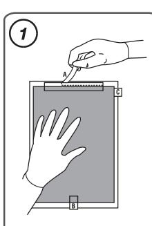
Place film, liner side down, onto LCD panel, and center within metal bezel. Holding film firmly in place with one hand, remove liner from tab 'A' and adhere tab A to metal bezel. Check film alignment; realign if necessary. Then place tab 'B', Scotch® Brand Tape on the top surface of the film.
