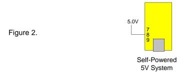
Figure 2 illustrates a typical USB self-powered configuration. A USB self-powered device gets its power from its own power supply and does not draw current from the USB bus.
