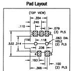
Tape Spec's: 24mm wide; 16mm pitch Reel Spec's: 15 inch reel (800 pieces per reel)
