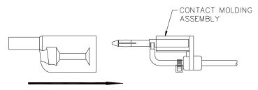
PUSH FIT ASSEMBLY INTO FRONT MOLDING, CHECK FOR PROPER LATCHING.
