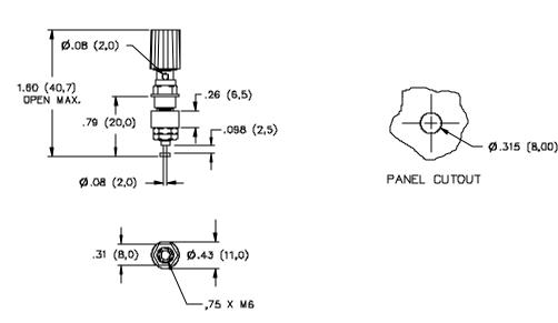
Recommended Maximuml Panel Thickness: .12" (3,0mm)
