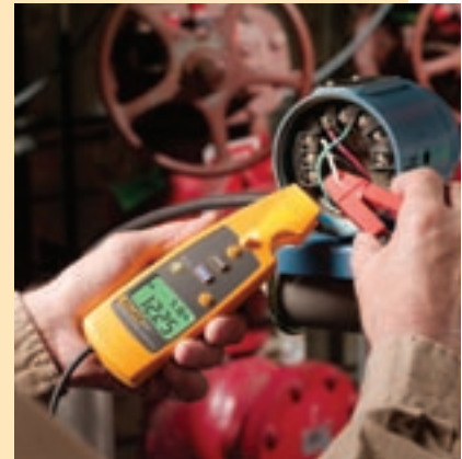
Detachable clamp used to measure 4 mA to 20 mA signals on transmitters without breaking the loop.
