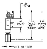
Center Contact: Brass, Gold Plated Impedance: 50 Ohms Insulation: ABS Molded to BNC (Male) and Binding Post Bodies, Color: Black Marking: "1296 POMONA" Binding Post: Body - Brass, Nickel Plated Insulated Thumb Knob -Polycarbonate, Color: One Black, One Red
