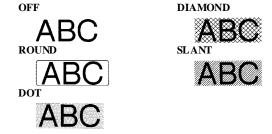
The default frame setting is **OFF**. When any setting other than **OFF** is selected, the **Frame** indicator on the right side of the display lights up.
