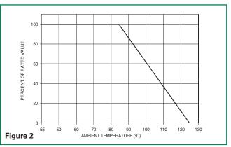
For applications exceeding 85°C ambient temperature, the peak surge current and energy ratings must be reduced as shown.
