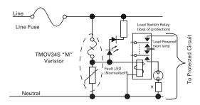
Please note: Indicator circuits are provided as a guideline only. Verification of actual indicator circuitry is the responsibility of the end user. Component values selected must be appropriate for the specific AC line voltage service and application.
