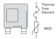
Note: MOVs are non-polarized passive elements
