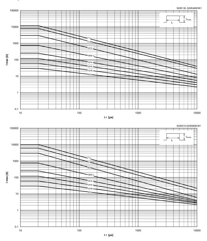
Derating curves (the specified current value in derating curve is the actual peak current throughout the varistor)
