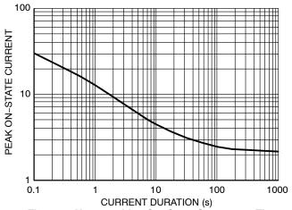
Figure 2. Nonrepetitive On-State Current vs. Time (I<sub>TSM</sub>)
