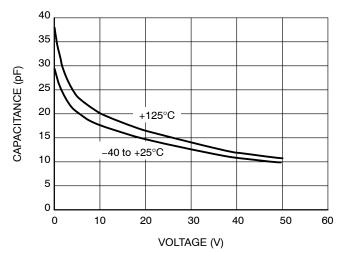
Figure 4. Capacitance vs. Off-State Voltage
