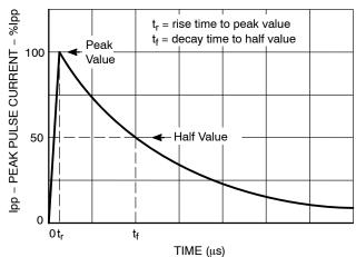
Figure 3. Nonrepetitive On-State Impulse vs. Waveform (I<sub>PPS</sub>)
