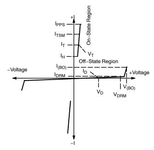
Figure 1. Voltage Current Characteristics of TSPD
