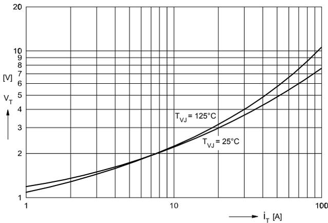
Fig. 3 On-state voltage
