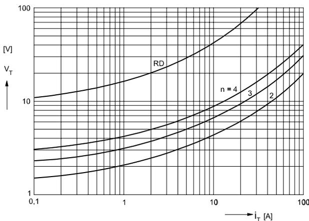
Fig. 7 On-state voltage at  $T_{VJ} = 125^\circ\text{C}$ .
