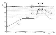
Typical values (solid line). Process limits (dotted lines). Vapour phase soldering.
