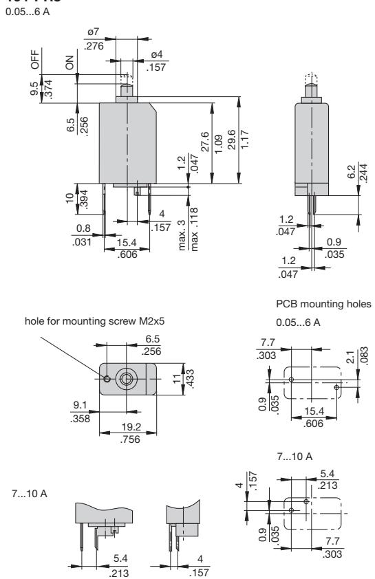
This is a metric design and millimeter dimensions take precedence ( $\frac{\text{mm}}{\text{inch}}$ )
