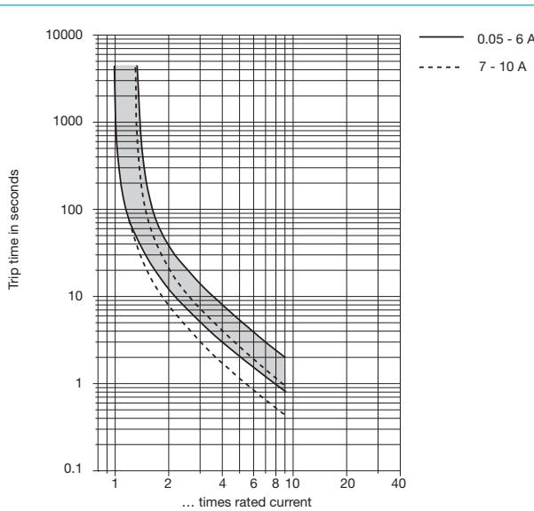
The time/current characteristic curve depends on the ambient temperature prevailing. In order to eliminate nuisance tripping, please multiply the circuit breaker current ratings by the derating factor shown below. See also section 9 – Technical information.
