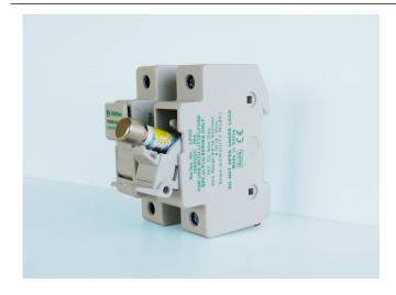
The LPHV midget fuse holder series is a touch-safe design providing protection to personnel when installing and removing fuses. The compact fuse holder mounts quickly onto 35 mm din rail decreasing panel layout and assembly time. It has been self-certified to stringent Littelfuse standards for applications upwards of 1000VDC when used with the Littelfuse SPF or FLU midget fuse series.
