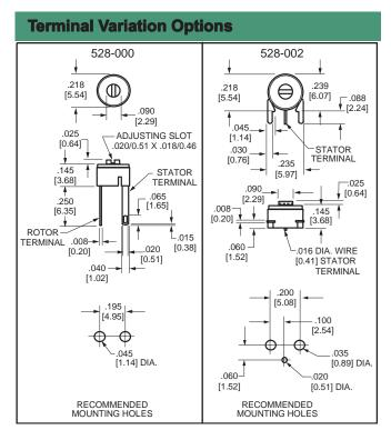
For dimensions  $\geq$  .126"/3.20mm, tolerance is  $\pm$ .015/0.38 For dimensions  $\leq$  .125"/3.18mm, tolerance is  $\pm$ .005/0.13
