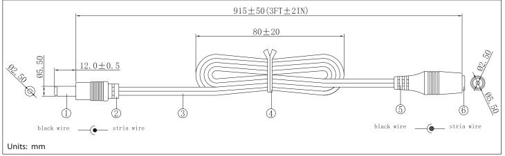
tolerance X: ±0.5 mm .X: ±0.3 mm .XX: ±0.05 mm applicable unless otherwise indicated in specification or on drawings
